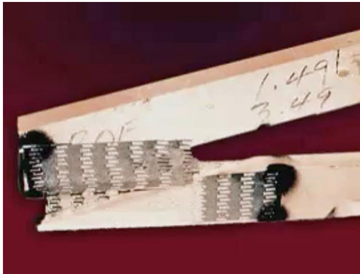
Plate failure due to shear forces
