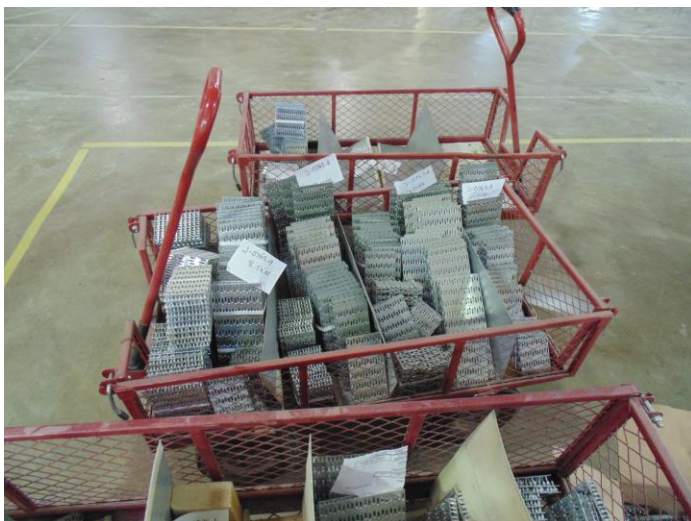
Left-Picking the exact plates for the trusses
