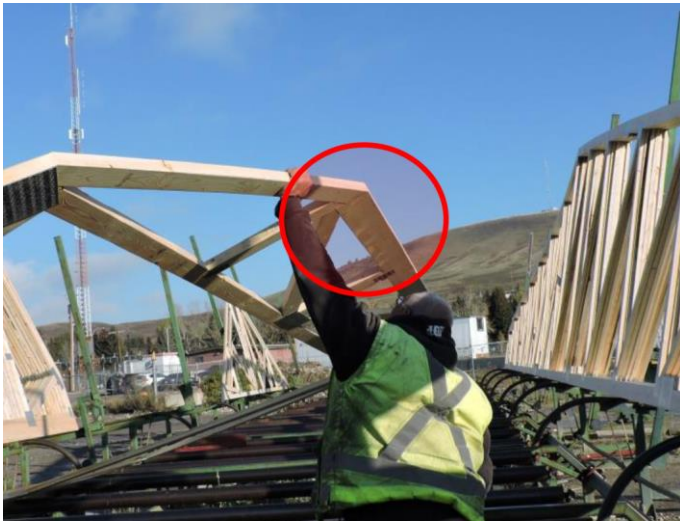
Checking the bottom side of the truss after pressing
