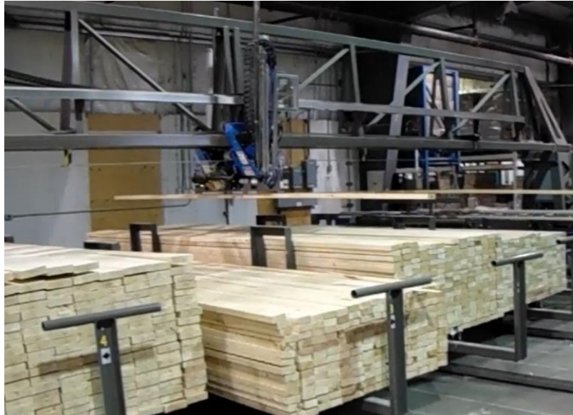
Automated Lumber Retrieval
