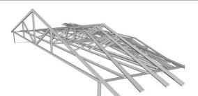
**21-Top Chord Bracing**-Permanent Top Chord Bracing is achieved via rigid sheathing or purlin strapping as designed by the building designer. The Top Chord may require permanent diagonal bracing as specified by the building designer.
