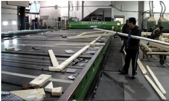
*The truss builder flips the board so that the crown is up.*
