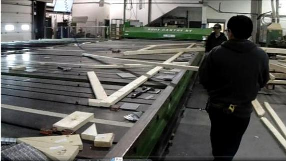
*The truss builder notices that the board has a crown and is going to flip it around.*
